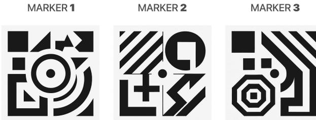
**Attention:** When placing the markers, make sure that at least one of them (or all) is positioned at a different height. This height variation helps the device track them more accurately.
