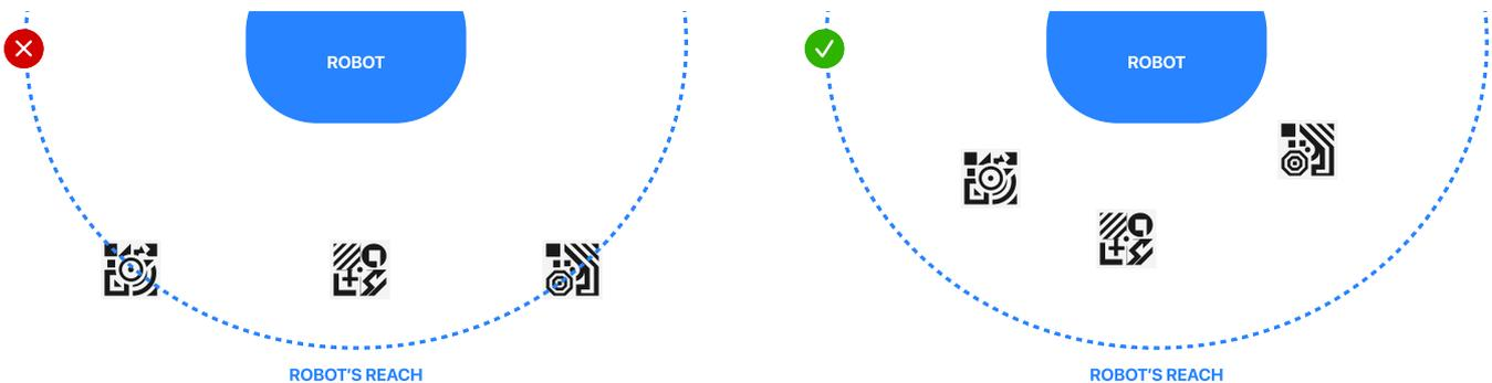
Once this is done, it's time to retrieve the robot's coordinates for each marker. To do this, manually move the robot to the center of each marker and input the corresponding coordinates into the app. Finally, select Done, and the calibration is complete.
